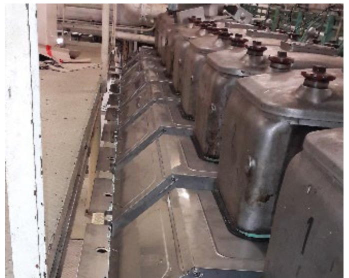
4. Fuel pump room covers to flip up to simplify the frequent inspections. Specially coated insulating components were developed for the indicator valves so that they can't absorb oil.
