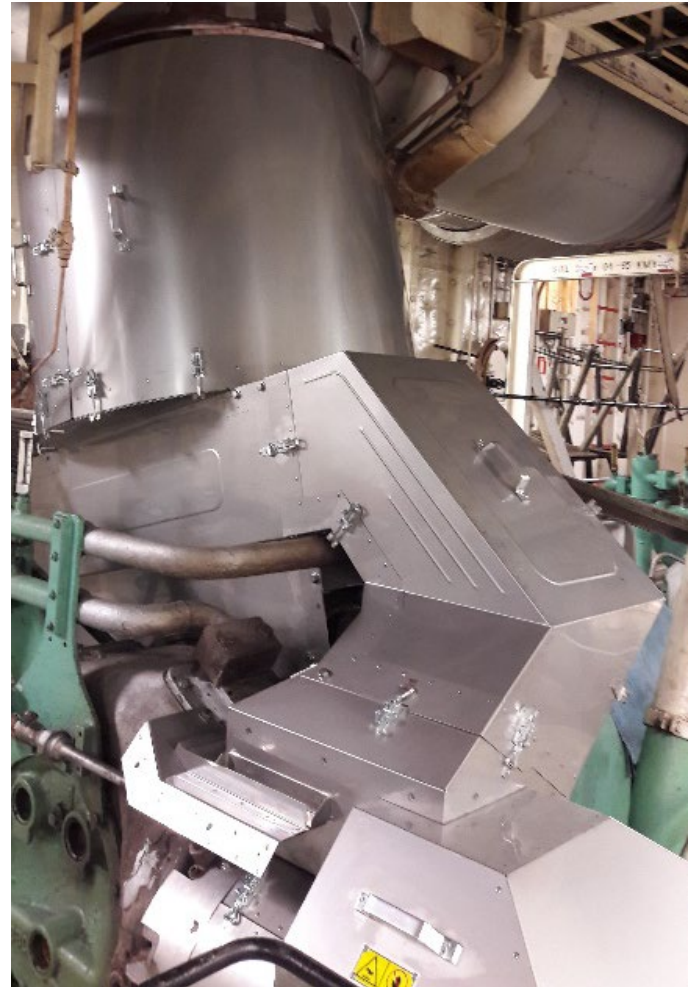
4. Fuel pump room covers to flip up to simplify the frequent inspections. Specially coated insulating components were developed for the indicator valves so that they can't absorb oil.
