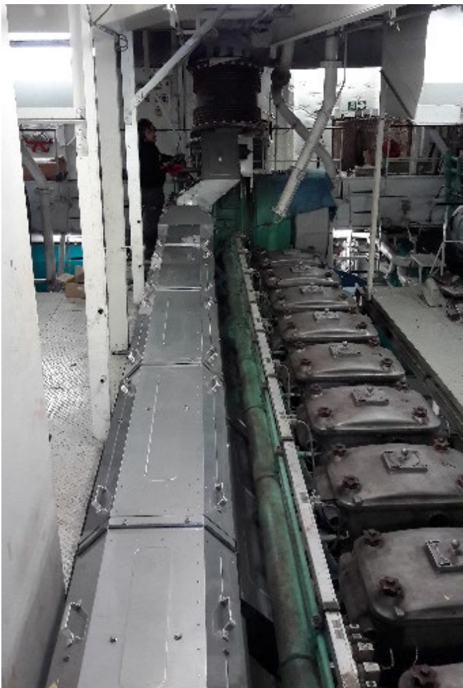
4. Fuel pump room covers to flip up to simplify the frequent inspections. Specially coated insulating components were developed for the indicator valves so that they can't absorb oil.
